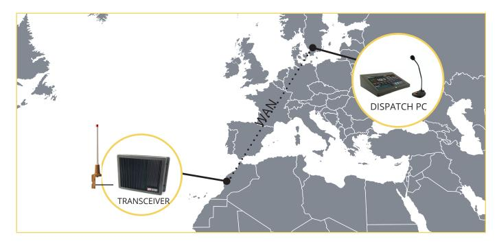
The system is a IP-network-based communication system (RTP protocol) that is controlled from a remote Operator PC. By using VCCS (**Vessel Communication Control System**) software, VHF & UHF voice communication equipment is integrated to a PC controlled by one operator.
